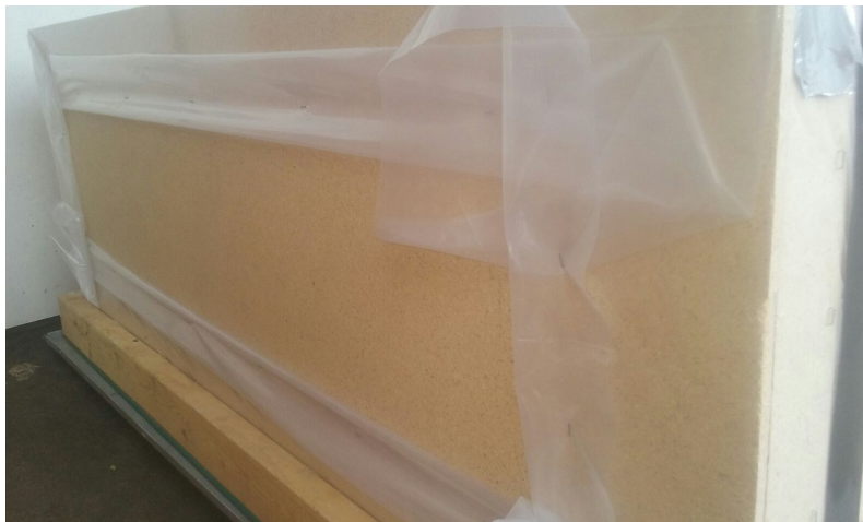
Figure 30: That's an outside look of how the plastic sheets works on one side, and then secured on the other side. Noting that will prevent it from getting contacted with the fiberglass resin.
