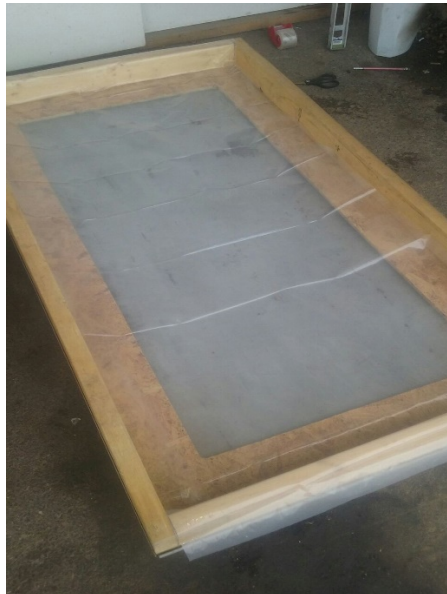
Figure 28: This is the top of the plug which has a hole cut out, so the child torso, head, and arms will be outside of the cart.
