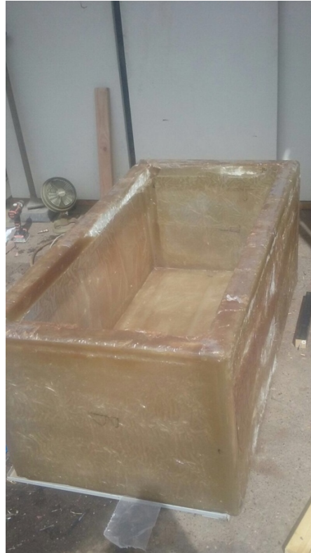
Figure 33: The molded exterior body of the cart.
